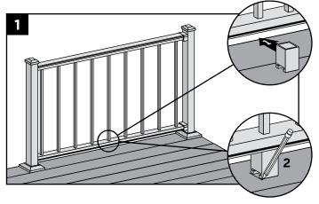
1. To ensure correct location, place foot block under center of bottom rail. Mark to provide placement location of base.
