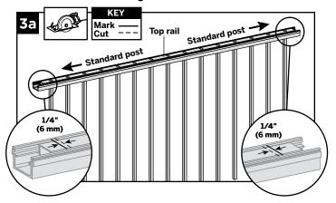
3a. Using a saw equipped with a non-ferrous metal blade, cut each end of top rail 1/4" (6 mm) shorter than mark to allow for fit into top rail brackets.
