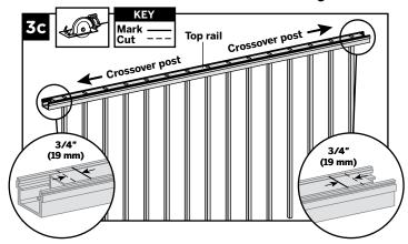
3c. Cut each end of top rail 3/4" (19 mm) **LONGER** than the mark to allow for fit into the crossover post bracket on each side.
