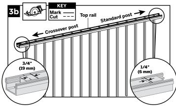
3b. Top rail must be cut differently on each side of the rail. Railing side that attaches to standard post should be cut 1/4" (6 mm) shorter than the mark to allow for fit into top rail bracket. Railing side that attaches to the crossover post should be cut 3/4" (19 mm) **LONGER** than the mark to allow for fit into the crossover post bracket.
