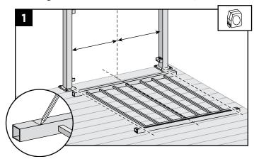
1. Position panel between posts and align with bottom bracket. Align center baluster with middle of span between posts (this will allow for equal spacing between end balusters and each post). Mark bottom and top rail at each end.
