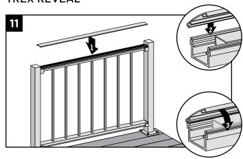
11. Attach upper rail cover to upper rail by aligning cover on one side of rail. Then starting from one end of rail, snap cover onto opposing slot working down length of rail. A **rubber mallet** may facilitate the fastening, using **GENTLE** tapping.
