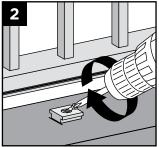
NOTE: Pre-drilling is recommended (1/8" [33 mm] drill bit) for attachment of base.
