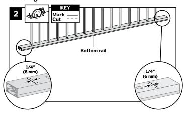
2. Using a saw equipped with a non-ferrous metal blade, cut each end of bottom rail and bottom rail insert 1/4" (6 mm) shorter than mark on each end to allow for fit into bottom rail brackets.
