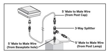
**NOTE:** If connecting a Reveal post cap light as well, a 3-way adapter and extra 5' Male to Male wire (not provided) can be used inside the post so that only one wire must be run through the hole in the base of the post (and post blocking). This is optional.
