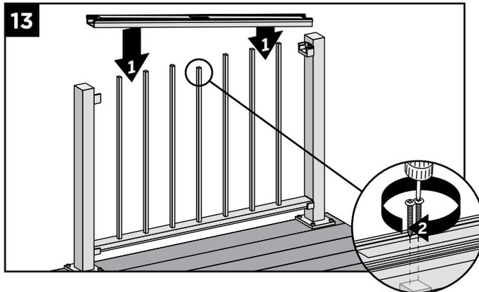
13. Working from one end of upper rail, snap balusters into upper rail working down length of rail. Fasten center baluster into center slot using two #8 x 1-1/4" (3.2 cm) screws (provided).
