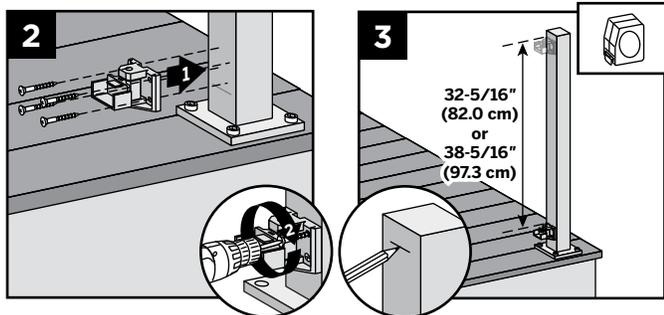
2. Center lower bracket on post **above** the marked line and attach using four self-tapping screws (provided).
