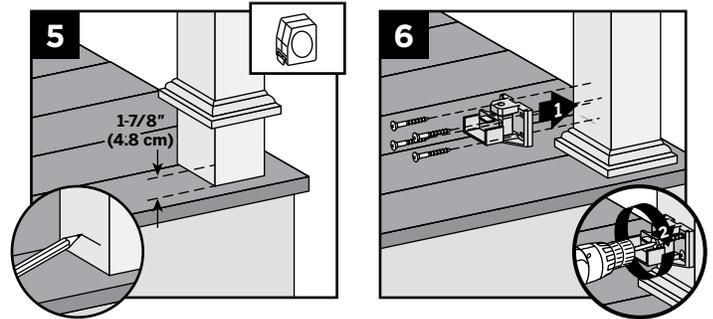
5. Measure 1-7/8" (4.8 cm) up from deck surface to bottom of bracket. Slide skirt up to allow for proper measurement, then push skirt back down onto surface of decking **BEFORE ATTACHING BRACKET**. Mark with light line.
