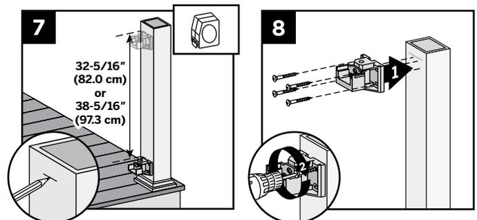
7. Measure up 32-5/16" (82.0 cm) for 36" (91.4 cm) tall railing or 38-5/16" (97.3 cm) for 42" (106.7 cm) tall railing from top of lower rail bracket. Mark with a light line.
