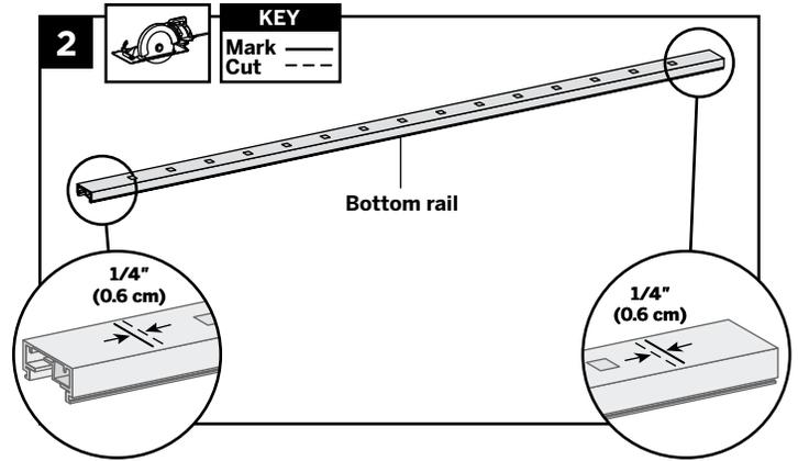
2. Cut each end of bottom rail 1/4" (0.6 cm) shorter than mark on each end to allow for fit into bottom rail brackets.
