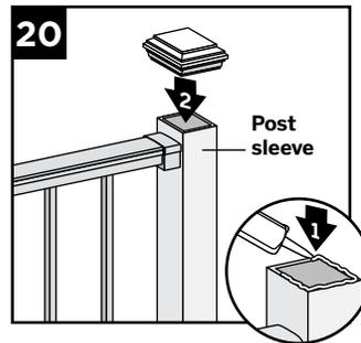
19. Attach post caps to Reveal posts (use of **rubber mallet** may be required for secure attachment).
