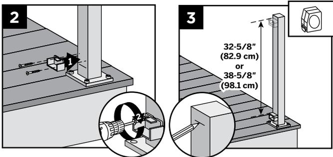
2. Center lower bracket on post **above** the marked line and attach using two self-tapping screws (*provided*).
