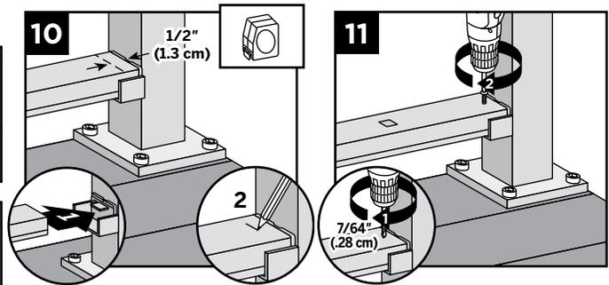
10. Set bottom rail into bottom brackets. Tabs on brackets will be inside of bottom rail (not shown when railing is attached). To ensure fit into tab, measure and mark 1/2" (1.3 cm) out from side of post.
