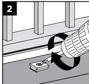
**NOTE: Pre-drilling is recommended (1/8" [0.32 cm] drill bit) for attachment of base.**
