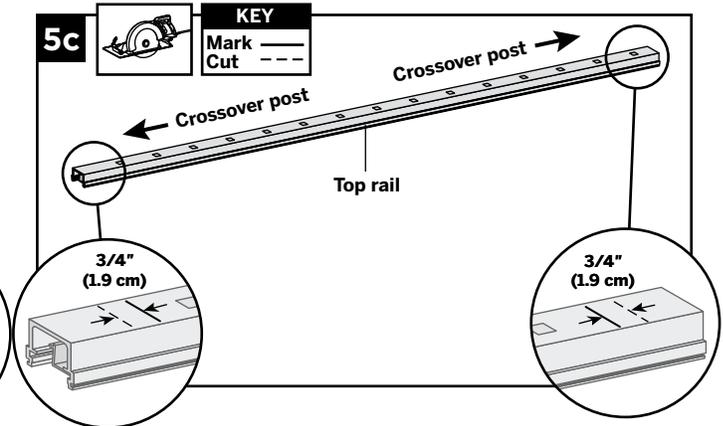
5c. Cut each end of top rail 3/4" (1.9 cm) **LONGER** than the mark to allow for fit into the crossover post bracket on each side.
