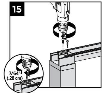
**NOTE: Pre-drilling is recommended (7/64" [0.28 cm] drill bit) for attachment of railing to post.**
