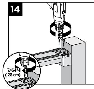
**NOTE: Pre-drilling is recommended (7/64" [0.28 cm] drill bit) for attachment of railing to bracket.**
