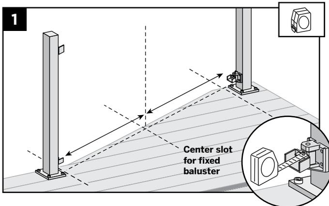
1. With brackets in correct swivel location, measure distance from inside of bracket to inside of bracket. ENSURE THAT BEFORE CUTTING, BALUSTERS HOLES ON BOTH BOTTOM AND TOP RAIL LINE UP. ALSO MAKE SURE CENTER BALUSTER SLOT IS AS CLOSE TO THE MIDDLE OF THE SPAN AS POSSIBLE. In some cases due to odd railing spans, the center baluster may need to be offset in one or the other direction to ensure there is enough room at both post locations for balusters to be placed.
