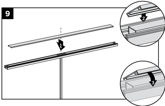
9. Attach "flat" bottom rail cover to bottom rail by first centering cover on bottom rail (this will allow gap on each end of bottom rail for placement into brackets). Align cover on one side of bottom rail in slot on side of rail. Then starting from one end of rail snap cover onto opposing slot working down the length of rail. In some cases, a **rubber mallet** may facilitate the fastening using **GENTLE** tapping.
