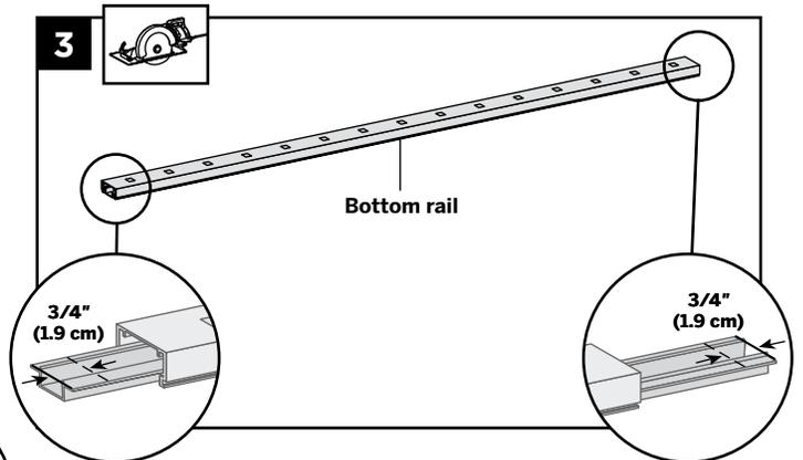
3. Slide rail insert out and cut 3/4" (1.9 cm) FROM EACH SIDE of insert, then slide back inside rail and center.
