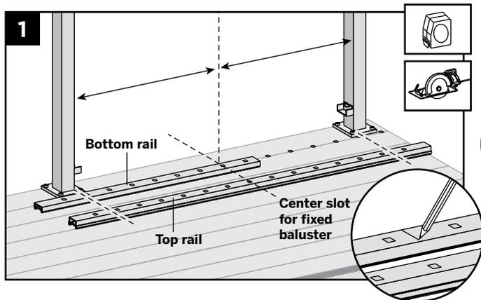
1. Position bottom and top rails between posts and align with bottom bracket. Align the center baluster slot in both rails with the middle of the span between posts.\* This will allow an equal number of baluster holes on each side of center slot. Mark bottom rail and top rail at each end (ensure both rails are centered between posts).
