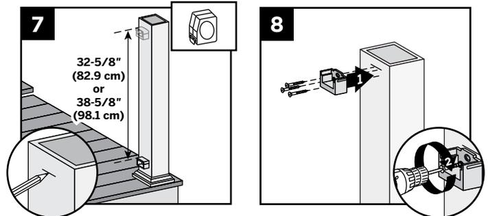
7. Measure up 32-5/8" (82.9 cm) for 36" (91.4 cm) tall railing or 38-5/8" (98.1 cm) for 42" (106.7 cm) tall railing from top of lower rail bracket. Mark with a light line.
