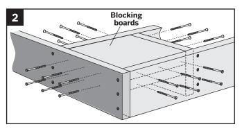
2. Install two 2" x 8" (5.1 cm x 20.3 cm) boards as blocking under post location. Securely attach blocking using a total of twenty-four 3" (7.6 cm) pressure-treated compatible screws (*not provided*).
