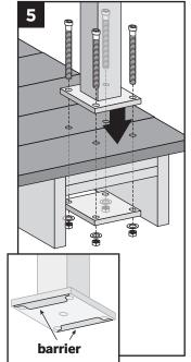
plate **MUST** be installed under the decking to ensure this will meet code compliance. *Reference SKU part number ALPOSTHWDECK for required hardware and aluminum plate.* (Consult local code official for more information on IRC Compliance.)
