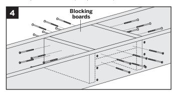
Install two 2" x 8" (5.1 cm x 20.3 cm) boards as blocking under post location. Securely attach blocking using a total of twenty-four 3" (7.6 cm) pressure-treated compatible screws (not provided). 5. **NOTE:** RIM JOIST REMOVED TO SHOW PROPER ATTACHMENT OF HARDWARE.
