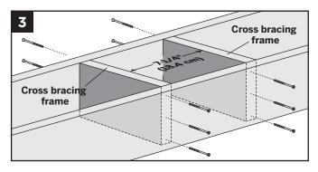
Install two 2" x 8" (5.1 cm x 20.3 cm) cross bracing frames in between joists at 7-1/4" (18.4 cm).
