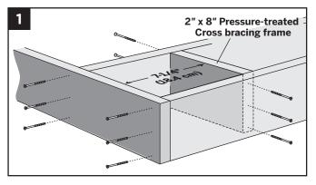
1. Install 2" x 8" (5.1 cm x 20.3 cm) cross bracing frame in between joists at 7-1/4" (18.4 cm). Attach a total of twelve 3" (7.6 cm) pressure-treated compatible screws (not provided).
