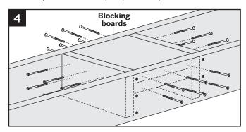
4. Install two 2" x 8" (5.1 cm x 20.3 cm) boards as blocking under post location. Securely attach blocking using a total of twenty-four 3" (7.6 cm) pressure-treated compatible screws (not provided).
