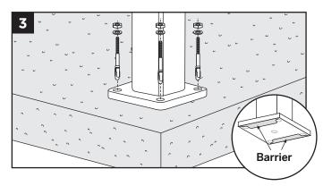
3. Insert the (2) stainless steel barrier stripes under the mounting bolt holes. Use appropriate shims if posts are not plumb. Secure post mount with the four expansion anchors, washers and nuts.
