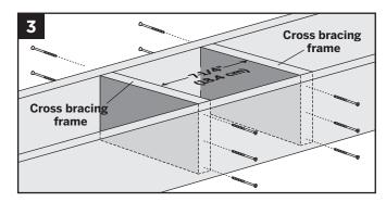
3. Install two 2" x 8" (5.1 cm x 20.3 cm) cross bracing frames in between joists at 7-1/4" (18.4 cm). Attach a total of twelve 3" (7.6 cm) pressure-treated compatible screws (not provided).
