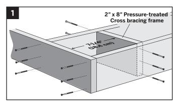
1. Install 2" x 8" (5.1 cm x 20.3 cm) cross bracing frame in between joists at 7-1/4" (18.4 cm). Attach a total of twelve 3" (7.6 cm) pressure-treated compatible screws (not provided).
