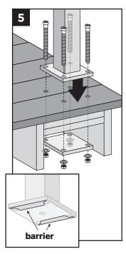
plate **MUST** be installed under the decking to ensure this will meet code compliance. Reference SKU part number ALPOSTHWDECK for required hardware and aluminum plate. (Consult local code official for more information on IRC Compliance.)
