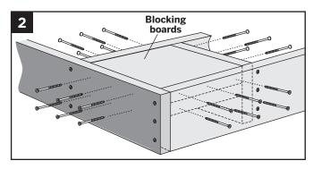
2. Install two 2" x 8" (5.1 cm x 20.3 cm) boards as blocking under post location. Securely attach blocking using a total of twenty-four 3" (7.6 cm) pressure-treated compatible screws (not provided).
