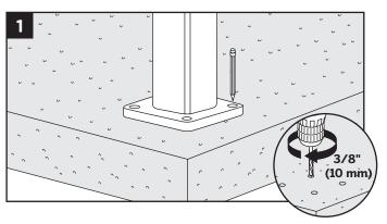
Using post as a template, mark locations of the four holes and drill into concrete at least 2-5/8" (66.7 mm) using a 3/8" (10 mm) masonry bit.
