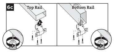
6c. At the lower post location for both top and bottom railing, attach the correct oriented bracket as shown. For TOP RAIL, the bracket would be attached to the side with baluster holes. For bottom rail, the brackets would be on the OPPOSITE SIDE of the baluster holes. Attach brackets using three #10 x 1" self-tapping screws (provided).
