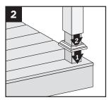
**NOTE:** Shims can be used to plumb post sleeves.
