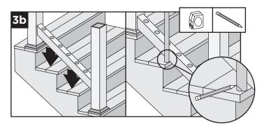
3b. Set bottom railing on nose of stair treads and set baluster at 90° on the outside of the railing, mark and measure the angle.
