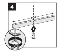
Cutting (see note below) and Inserting Aluminum Baluster Adaptor Strip into Bottom Rail
