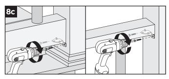
8c. Install both bottom and top brackets on each side to post using two #8 x 2" screws (*provided*). For best results, set drill to low speed when installing these screws.
