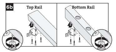
6b. At the upper post location for both top and bottom railing, attach the correct oriented bracket as shown. On the TOP RAIL, attach the bracket to the side with baluster holes. On the BOTTOM RAIL, attach the bracket to the **OPPOSITE SIDE** of the baluster holes. Attach brackets using three #10 x 1" self-tapping screws (*provided*).
