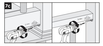
7c. Install both bottom and top brackets on each side to post using two #8-10x2" wood screws (provided). For best results, set drill to low speed when installing these screws.
