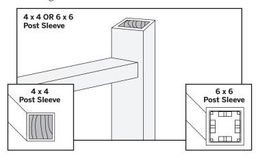
» Both 4" x 4" (102 mm x 102 mm) or 6" x 6" (152 mm x 152 mm) post sleeves work well for angles up to 45 degrees. Bottom rail brackets may need to be slightly offset to one side in order to fit properly to hold rail in
