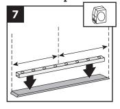
8. Secure deck board to Enhance top rail with #8-3/4" truss-head self-drilling screws (not provided) approx. every 16" on center. Screws are to be installed inside of the baluster holes into the decking board. **DO NOT** overtighten.
