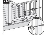
NOTE: To help stabilize railing section use a quickgrip clamp (or other type of clamp) and clamp the first baluster to post sleeve.
