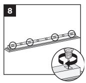
**NOTE:** A long drill bit will be required to fit inside the baluster holes.
