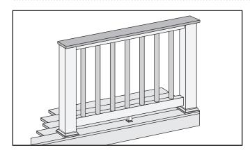
**Important: ONLY** use with pressure treated 4 x 4 post (3.5" nominal square) and 4" x 4" (102 mm x 102 mm) post sleeve. Trex Post Mounts or Joist Mount Posts cannot be used with Enhance Cocktail railing.
