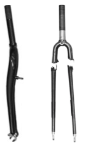
Figure 1. Overloaded forks: metal fork on left bent when overloaded. Carbon fiber fork on the right broke at a much higher load, but completely separated.
