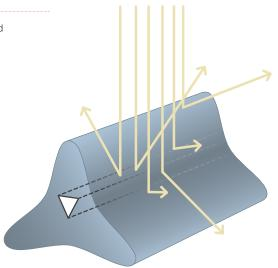
The Power of the Triangle: The shape and placement of the fiber's central hollow core delivers optimal light refraction while preserving color clarity.
