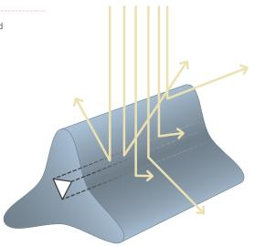
The shape and placement of the fiber's central hollow core delivers optimal light refraction while preserving color clarity.
