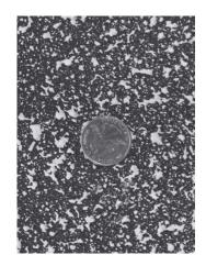
Proper Spray Pattern using US quarter for size comparison.
