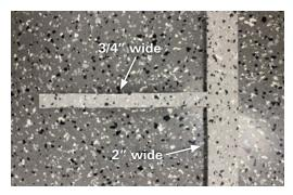
Take one tile and create a Tile - T this is used to measure from the top of the cove cap to the edge of the installed tile.
