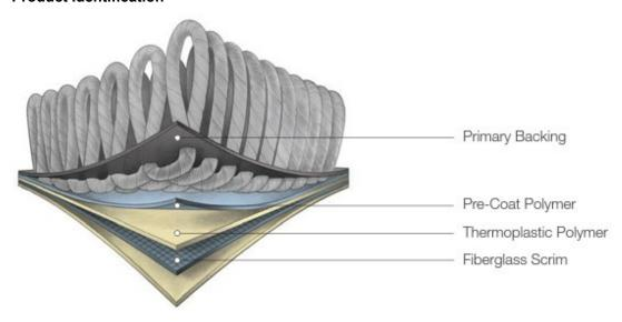
EcoFlex™ NXT is a modular carpet tile consisting of a nylon face fiber tufted into a primary backing; precoated with an acrylate polymer to lock the tufts into place; back coated with polyolefin polymer and fiberglass scrim for stability.
