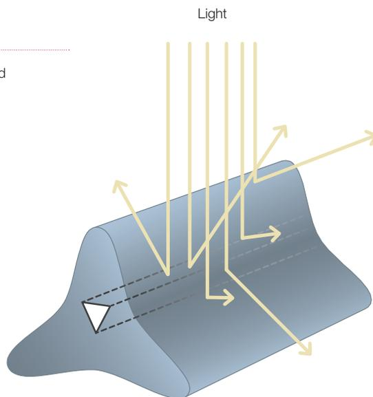
The Power of the Triangle: The shape and placement of the fiber's central hollow core delivers optimal light refraction while preserving color clarity.
