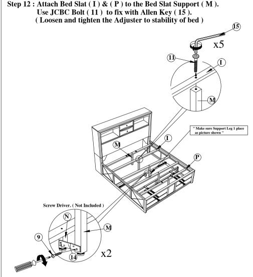
STEP 13 : Attach Z-Bracket (14) to the Bed Slat Support (M) and Support Leg 2 (N).Use Panhead Screw (9) and tighten with screw driver (not included)
