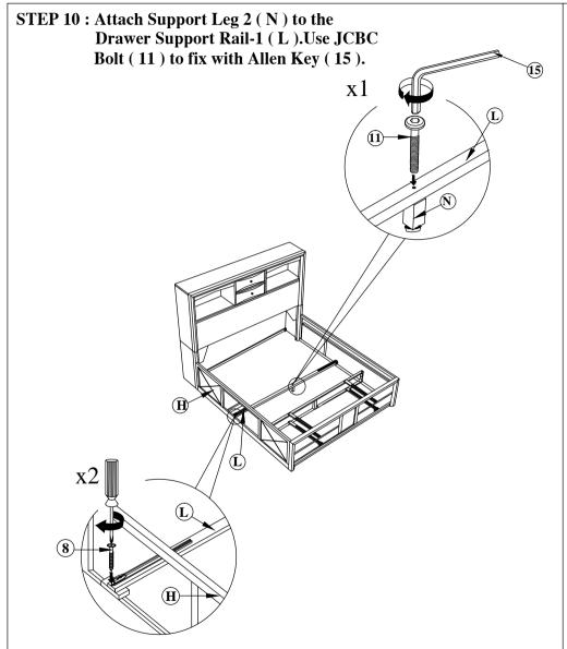
STEP 11 : Attach Drawer Support Rail-1 ( L ) to the Side Rail ( H ) using Csk Screw ( 8 ) and tighten with Screw Driver.( Not Included )
