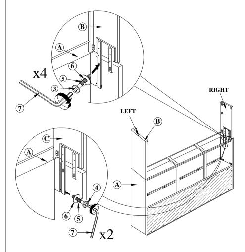
STEP 2 : Attached and tighten the Headboard Leg L/R (B) to the Headboard (A).Insert Spring Washer (5) Flat Washer (6),use JCBC Bolt (4) to fix with Allen Key (7).
