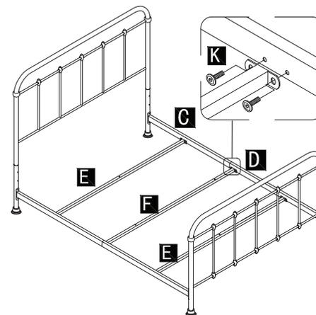
**Step 5.** Attach the center legs to the slats (E) & (F) with bolts (L). Tighten with Allen wrench (J).
