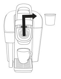
**6.** Remove all parts as shown below and clean and sanitize thoroughly per Clean & Sanitizing procedures on page 4.
