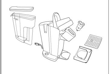
**7.** Wipe interior of the puncture mechanism with a clean cloth dipped in Urnex<sup>®</sup> Complete Café sanitizer.
