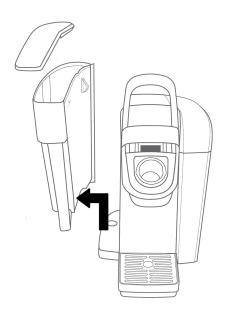
**4.** Locate door on rear of brewer and remove drain line. Drain water from brewer into a water-tight container.
