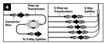
4. Connect opposite end of male connector wire cable to female end on Step-up Transformer. If using more than one spotlight, use 5-way splitter on Step-up Transformer, making sure that each spotlight is utilizing its own 36V Step-up Transformer. Wire the Step-up Transformer or 5-way splitter to the 5A main transformer.
