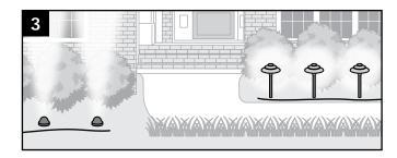
Run all wires from the power source locations to the lights on top of the soil, being mindful to leave slack. Pay special attention if using separate circuits with independent dimmers (grouping lights by type is recommended).
