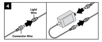
4. Connect all lights. Wire the optional dimmer (recommended) between the main 20' (6.1 m) transformer to male lead and the transformer for each circuit. Ensure connections (including splitters), fixtures, and power sources all work properly.
