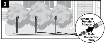
3. Connect opposite end of female adaptor to male connector wire. Choose appropriate length wire based on your needs. Run all wire on the surface back to the location of the power supply.
