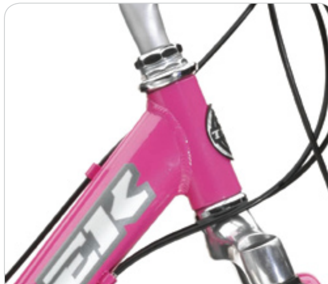
FIGURE 1 | No gusset; if model is listed on the chart to the left, the bicycle is recalled.
