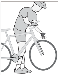
FIGURE 1.4 Test for loose condition
