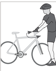
FIGURE 1.3 Function test for the handlebar and stem
