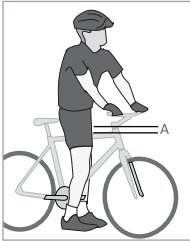
FIGURE 1.1 A = Minimum standover clearance 1" (25 mm) for most bicycles 2-3" (50-75 mm) for mountain bicycles
