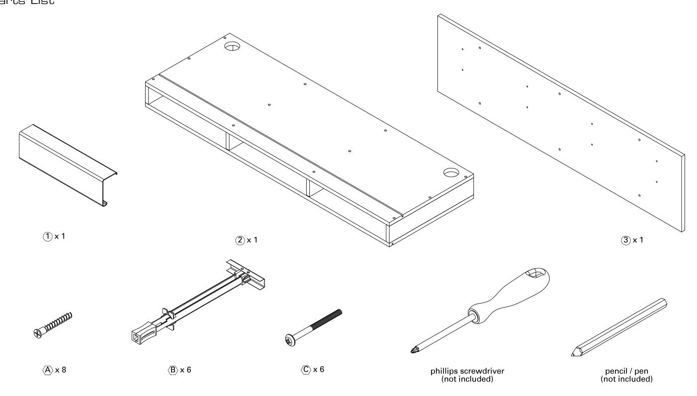
Use part (3) to locate placement of the Wall Mounted Desk. Check to ensure part is level. Mark with pencil the location of six holes to be drilled. Drill a 1/2" hole at the six shown locations on the next page.
