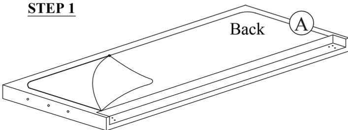
Open the zipper stitched on the back of Headboard (A) and take out the Footboard (D) from the storage space of Headboard (A).
