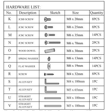
Note: Straight Allen Key (U) & (V) are for use with a power drill.
