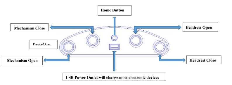
Care should always be taken to assure there is nothing in the path of the mechanism before and during operation
