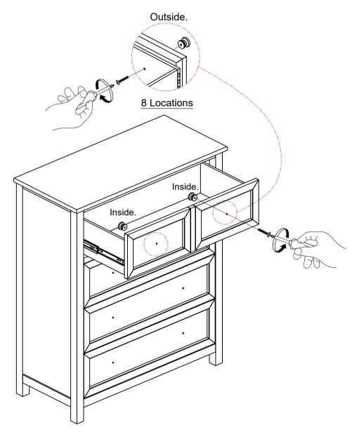
Unscrew the handle from inside of drawer and assemble it out side.
