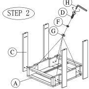
Note:Do not fully install or tighten Bolts until after Shelf is assembled.
