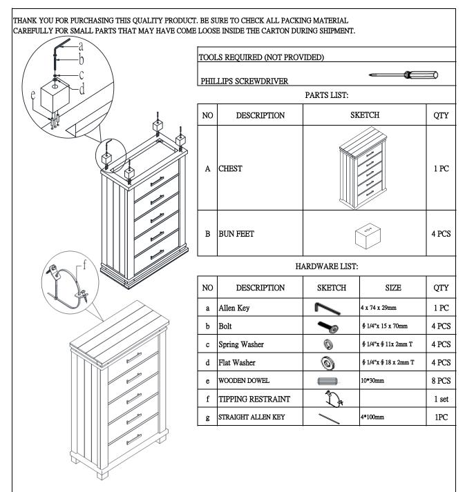
STEP 1: Lay the chest (A) up side down on a soft surface. Insert wooden dowel (e) to the bottom of chest (A). Attach bun feet (B) by using allen key (a), bolt (b), spring washer (c), flat washer (d).
