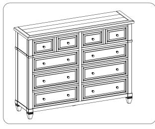
STEP 1: Put the case upside down on a soft surface, Attach the legs and support leg to the bottom of case by using 8 bolts(A), lock washers(B) and flat washers(C). Return the case to the upright position.
