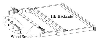
STEP 2: Attach the wood stretcher to the legs by using 4 bolts(B), lock washers(D) and flat washers(E).
