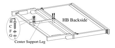
STEP 4: The side rails may be used on either side. Arrange the side rails so the slat bearers are in UPPER POSITION prior to attachment in STEP 5.
