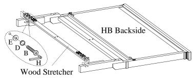
STEP 2: Attach the wood stretcher to the legs by using 4 bolts(B), lock washers(D) and flat washers(E).
