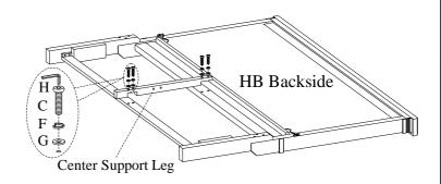
STEP 4: The side rails may be used on either side. Arrange the side rails so the slat bearers are in LOWER POSITION prior to attachment in STEP 5.
