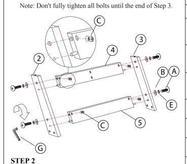
Note: Don't fully tighten all bolts until the end of Step 3.
